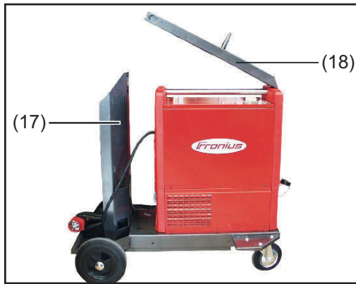
Fitting the wirefeeder mount
