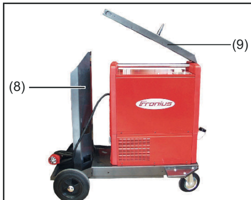
Removing the wirefeeder mount
